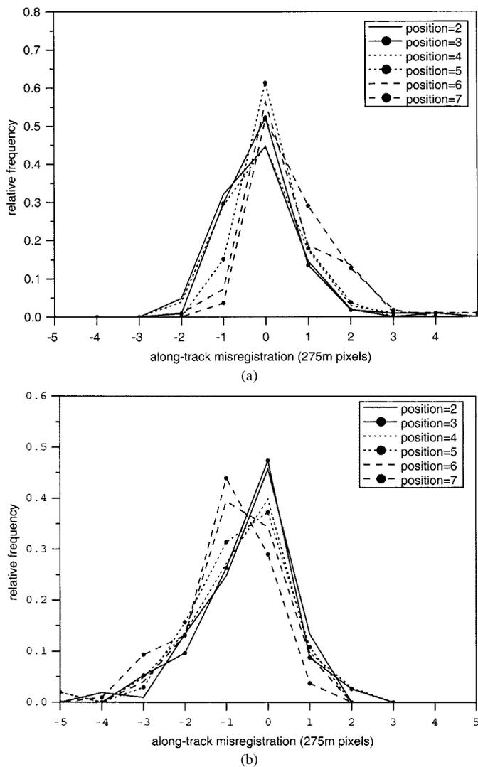
Fig. 6. Retrieved misregistration for (a) Df and (b) Da cameras for version 6 of the CGM. Combined misregistration distributions for several orbits are shown for six equally spaced domains across the swath.
