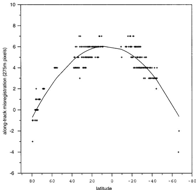
Fig. 4. Retrieved misregistration for the Da camera for version 4 of the CGM versus latitude. Results shown are for a single domain (across-track position = 7) gathered across multiple orbits. The solid line is a second-order polynomial fit to the data.
