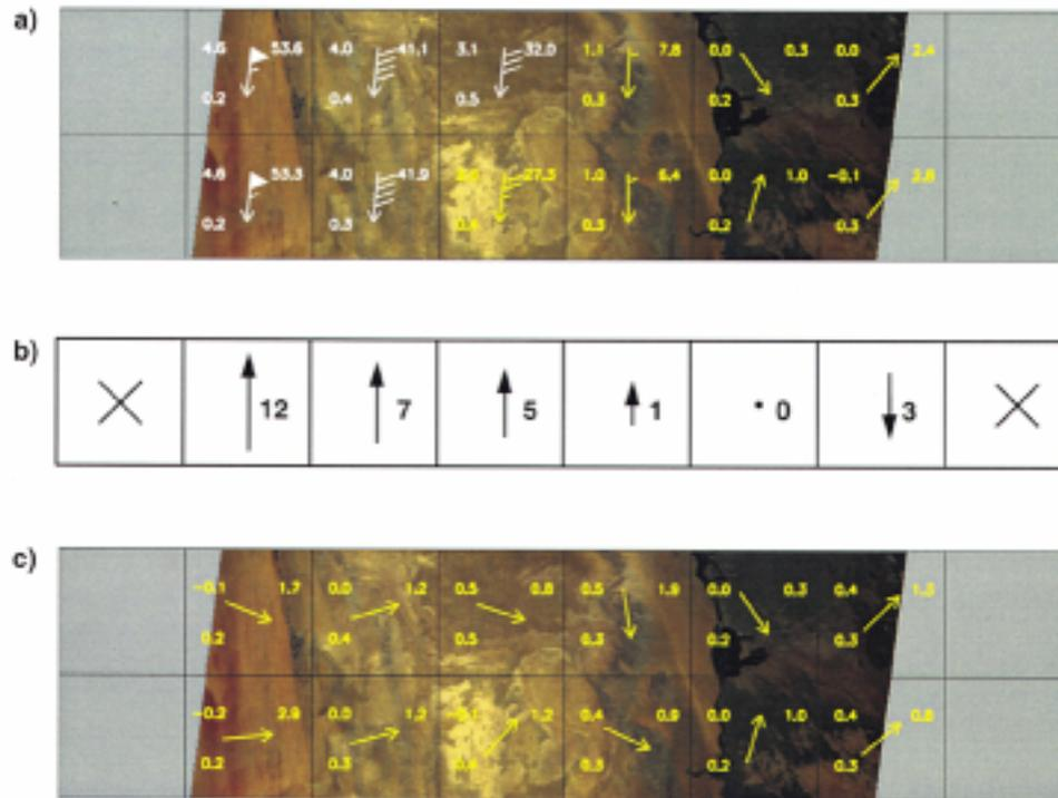
Fig. 5. Registration correction with the “zero-wind” method for path 175, orbit 1660, block 71. The area shown is just to the northeast of Nasser Lake, Egypt, with north pointing to the top of the image. (a) Wind retrievals without correction. (b) Df camera along-track correction (in 275-m pixels) as a function of cross-track position. (c) Wind retrievals with the correction given in (b).
