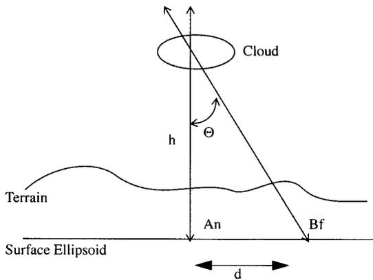
Fig. 1. MISR viewing geometry for the An and Bf cameras.
