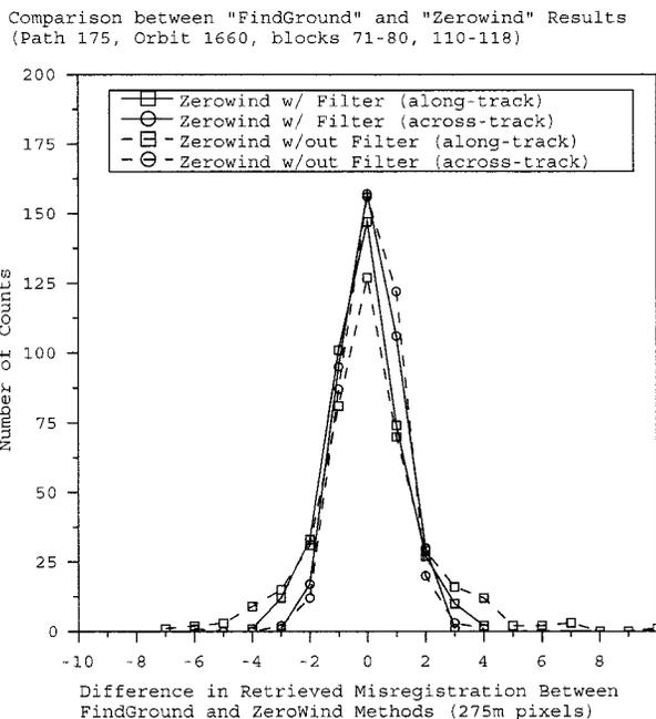
Fig. 2. Comparison of the find-ground and zero-wind methods for path 175, orbit 1660. A histogram distribution of the differences between the two methods are shown, with separate statistics being gathered for the Df and Da cameras in both the along- and across-track directions.
