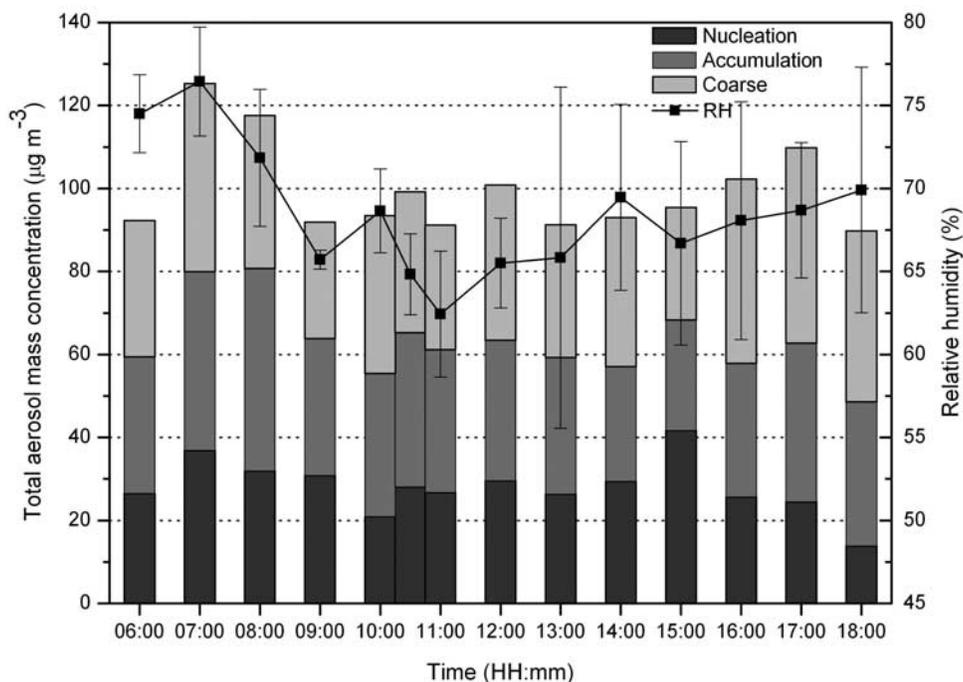
**Figure 6.** Diurnal variation of hourly mean total size-segregated near-surface aerosol mass concentration ( $\mu\text{g m}^{-3}$ ) and relative humidity (%).
