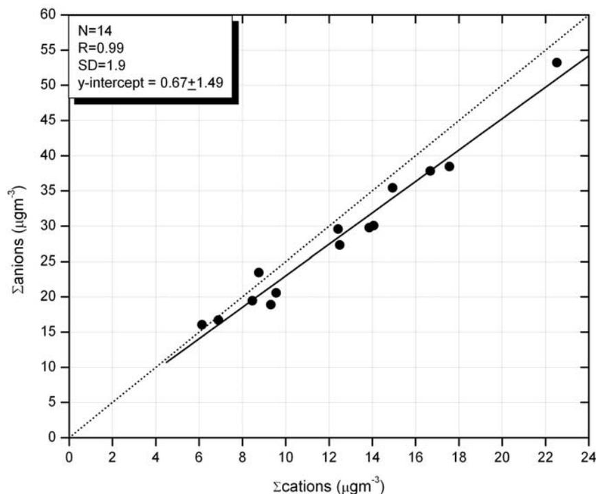
**Figure 11.** Ion balance between  $\Sigma$  cations and  $\Sigma$  anions representing quantitative characterization of water-soluble ionic species in aerosols during May–August 2005.
