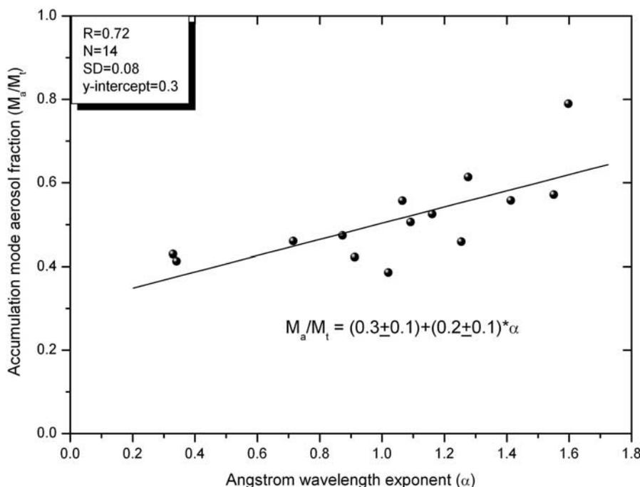
**Figure 8.** Scatterplot of  $M_a/M_t$  along with Angstrom wavelength exponent ( $\alpha$ ) for the days of simultaneous observations.
