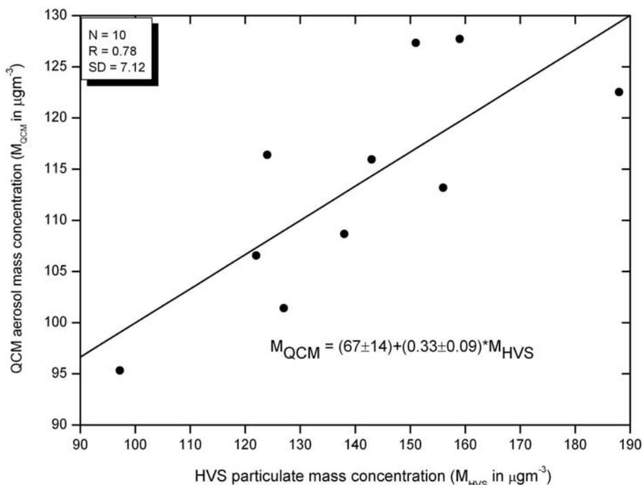
**Figure 9.** Scatterplot of QCM measured total aerosol mass concentration ( $\mu\text{g m}^{-3}$ ) along with the HVS measured aerosol particulate mass concentration ( $\mu\text{g m}^{-3}$ ).
