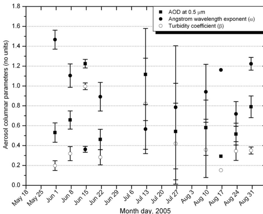
**Figure 3.** Time series of average values of AOD at 0.5  $\mu\text{m}$  measured during the days of observation with the variation of Angstrom wavelength exponent  $\alpha$  and Angstrom turbidity coefficient  $\beta$  estimated from the daily mean AOD spectra.
