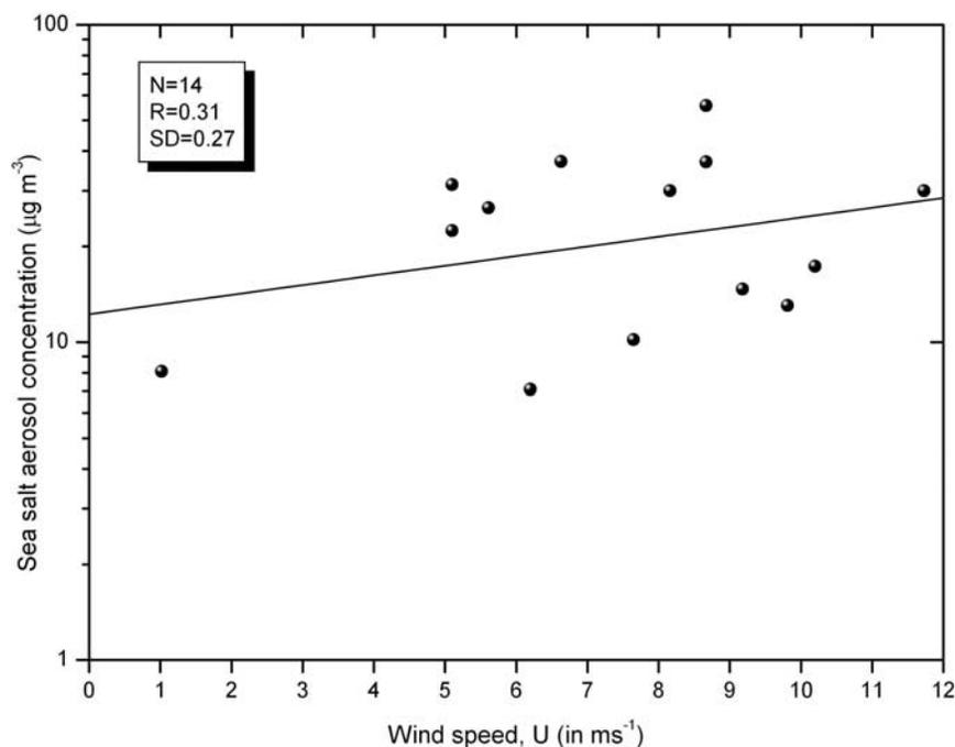
**Figure 13.** Dependence of sea-salt aerosol mass concentration ( $\mu\text{g m}^{-3}$ ) on the prevailing wind speed ( $\text{ms}^{-1}$ ) over Visakhapatnam during the summer monsoon season (May–August 2005).
